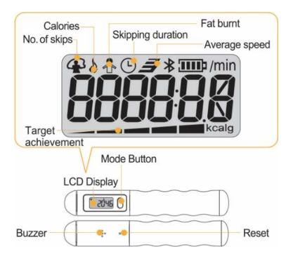
Mode Button: Press to switch between different modes or press and hold to initiate pairing. **Modes**
